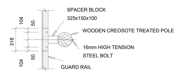
DETAIL OF PLACING AND MOUNTING
